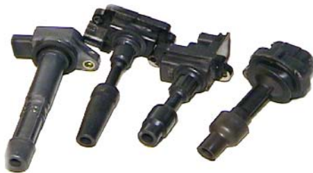
Coil on Plug (COP) or Coil near plug (CNP)
