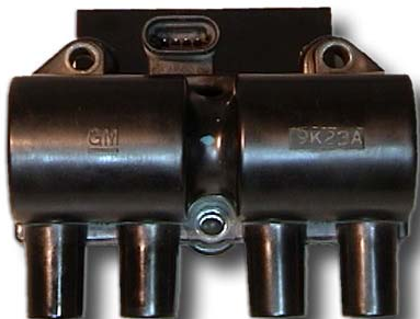
Double ended Coil on plug (DECOP)
